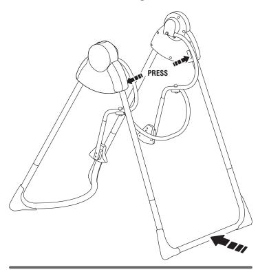
• Press the button on each housing and push the rear legs toward the front legs. Stand the frame against a wall for storage.
